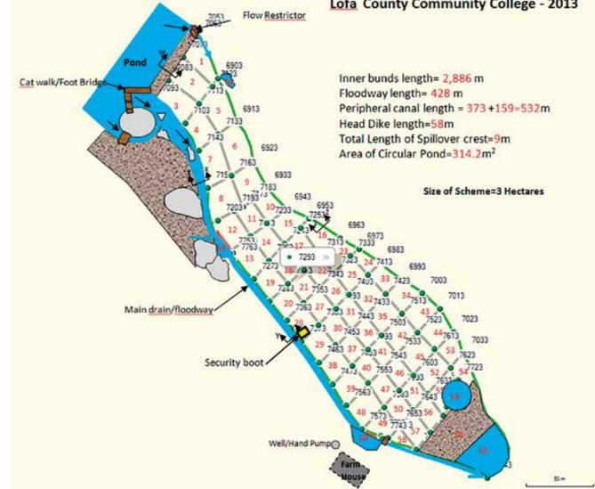
Fig. 13 A detailed swamp layout prepared with the help of a GPS data inserted into Google Earth image
