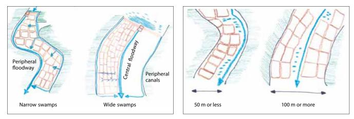
Fig. 12 Selection for Positioning of Floodway: Peripheral or Central Rain-fed scheme with floodway only Irrigation scheme with supply canals
