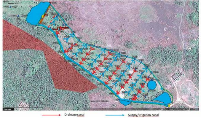
Fig. 14 A lay-out prepared with a print-out from Google Earth and hand-drawings with color pens
