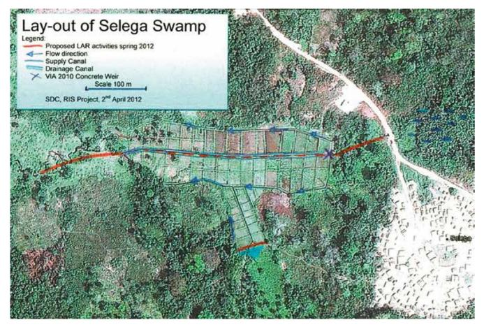
Fig. 15 A swamp layout prepared with a print-out from Google Earth and hand-drawings with color pens
