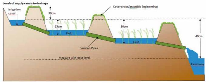
Fig. 11 Levels and Drops between Peripheral Canal and Floodway
