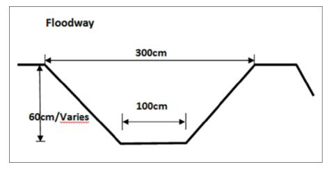
Fig. 20b Dimensions of floodways
