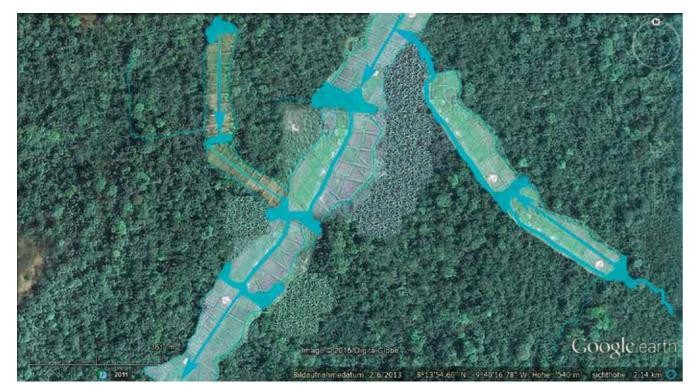
Fig 8 An idealistic landscape (photomontage) with lowland farming, swamp edge cultivation and preserved forests in the uplands. The irrigation schemes are all equipped with a retention pond at the intakes and Head dikes, which reduces run-off during storm events.
