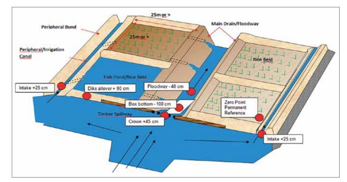
Fig. 10 Critical Levels at Head Dike an Intakes to Peripheral Canals
