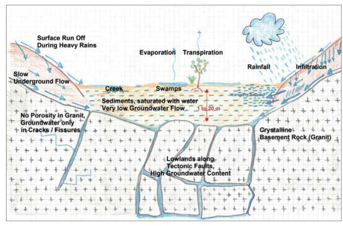
Fig. 4 Cross Profile of Lowland with Surface and Underground Flow of Water
