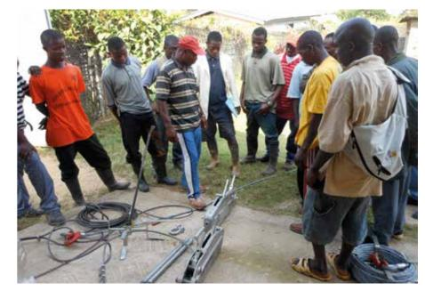
Fig. 17 Explaining the cable pulling device "Come Along" for tree de-stumping
