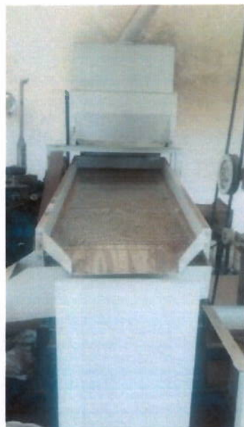
Photo 24: Motorised rice grader (capacity : 7-8 tonn/day)
