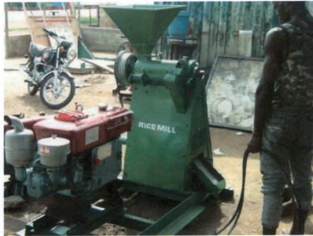
Photo 20: Small scale improved rice mill (type Enguelbert; with winnover)
