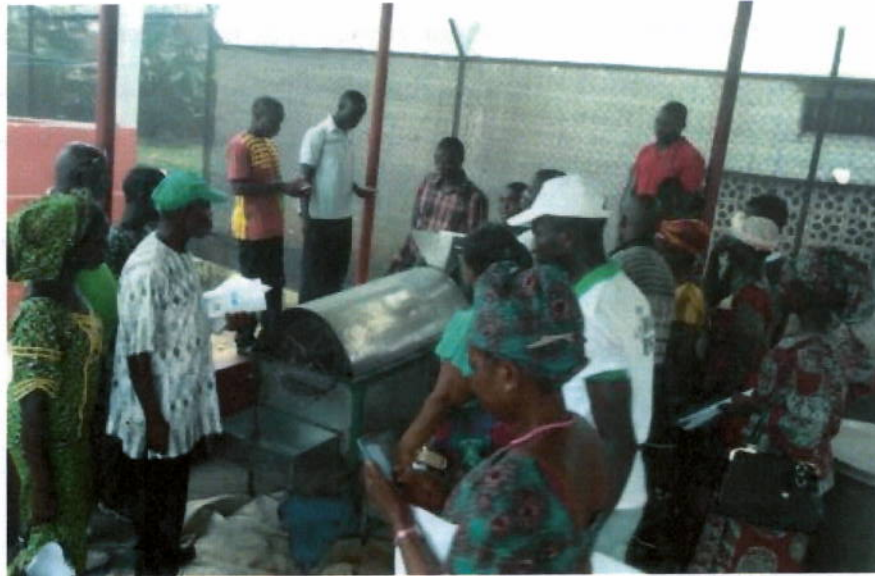
Photo 23: Manual mill rice grader (capacity 350-400 kg/h; 3 tonn/day)
