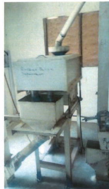
Photo 24: Motorised rice grader (capacity : 7-8 tonn/day)
