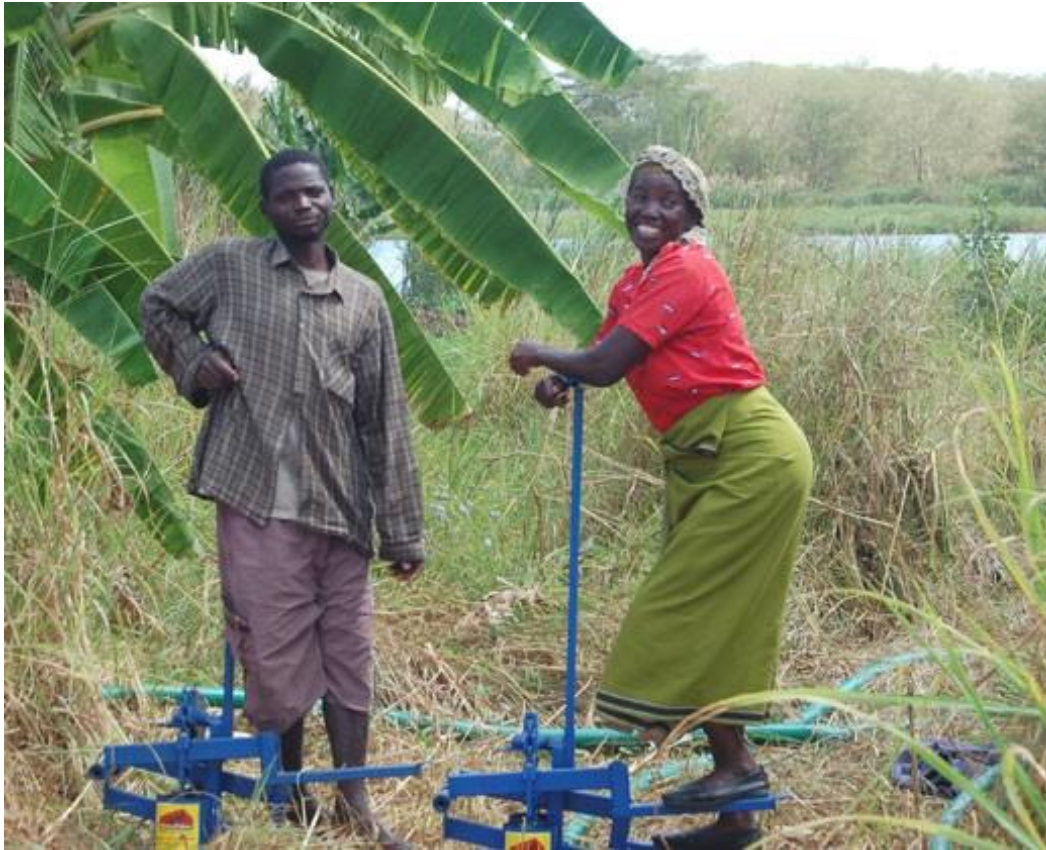
Figure 2: Foot pump irrigation unit which will be similarly fabricated in CARI under the project 2
